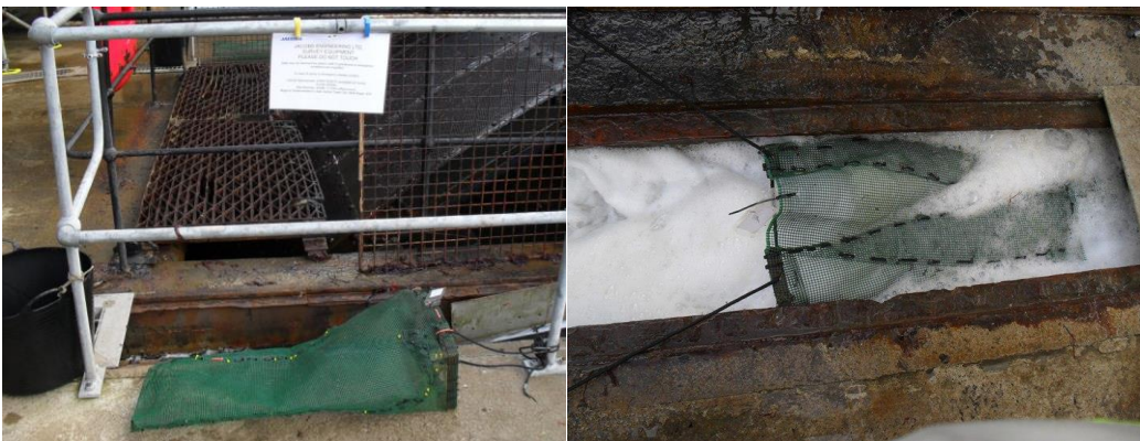
Figure 2.1 : An impingement-sampling basket about to be deployed (left) and a basket sampling in the drum screen wash channel (right).
