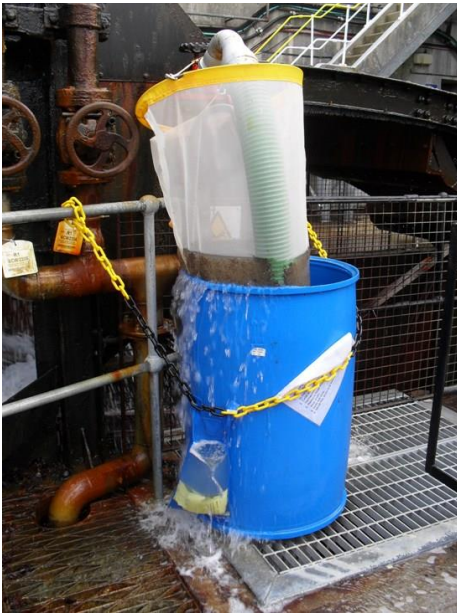
Figure 3.2 : Photograph showing the operation of ichthyoplankton entrainment sampling.
